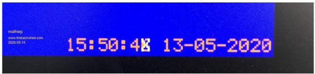
Note how the "X" appears to have overwritten the brown seconds units but the seconds are still incrementing underneath and pixels that are not covered by the "X" show normally.
