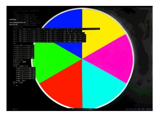
As explained earlier, 8-bit colour modes use a lookup table to convert from a single byte of information to the RGB565 pixel that will be displayed. In the CMM2 firmware the 8-bits are treated as a RGB332 pixel and are mapped to the most appropriate RGB565 value.
