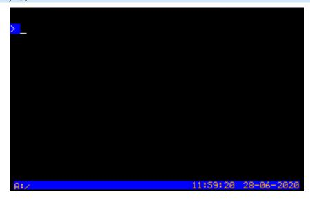
Check out the RGB function in the user manual. We have asked the system to clear the screen but to use a non-transparent black. Valid transparency values are from 0 to 15 where 15 is a solid colour. However, the default background colour is fully transparent black so the characters associated with the command prompt and the status line still show the blue colour.
